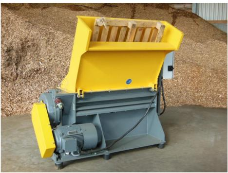
The manually fed pallet chipper SPE 1300 has been constructed specifically for shredding pallets and wood waste to high quality wood chips.
